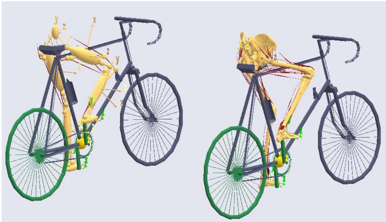
Figure 4. A typical example of a structured model: The two bicycles are identical applications within the same model and are combined with a simple, 2-D lower extremity and a more complicated 3-D lower extremity respectively.
